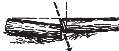
MAKE ANGLED CUT WHEN ONE SECTION MAY SETTLE AGAINST ANOTHER. KEEP BODY OUT OF BAR/CHAIN PATH!
